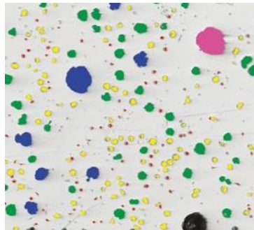
Ductile cast iron showing nodular graphite
